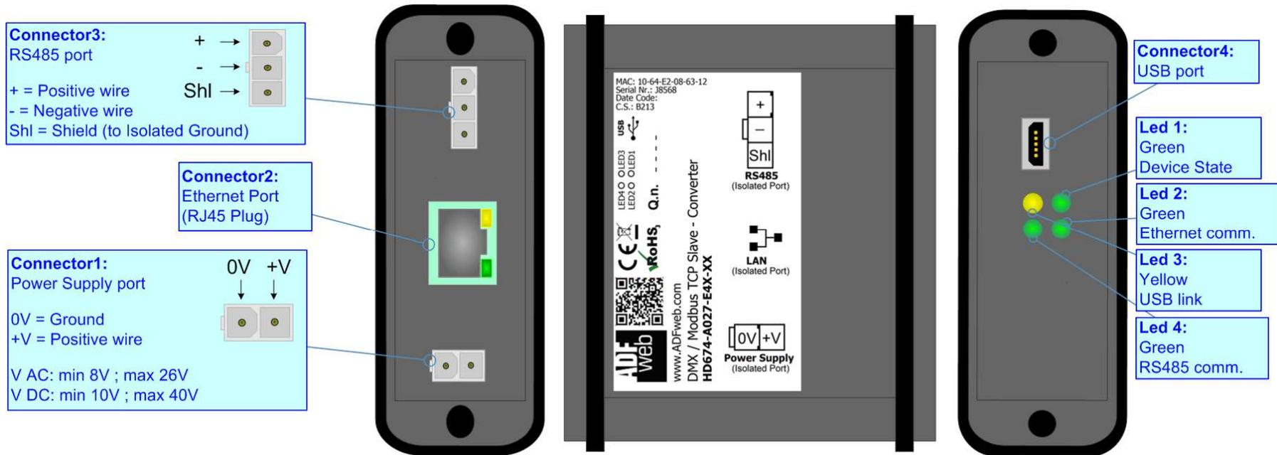
Figure 1a: Connection scheme for HD674-A034-E4x-xx
