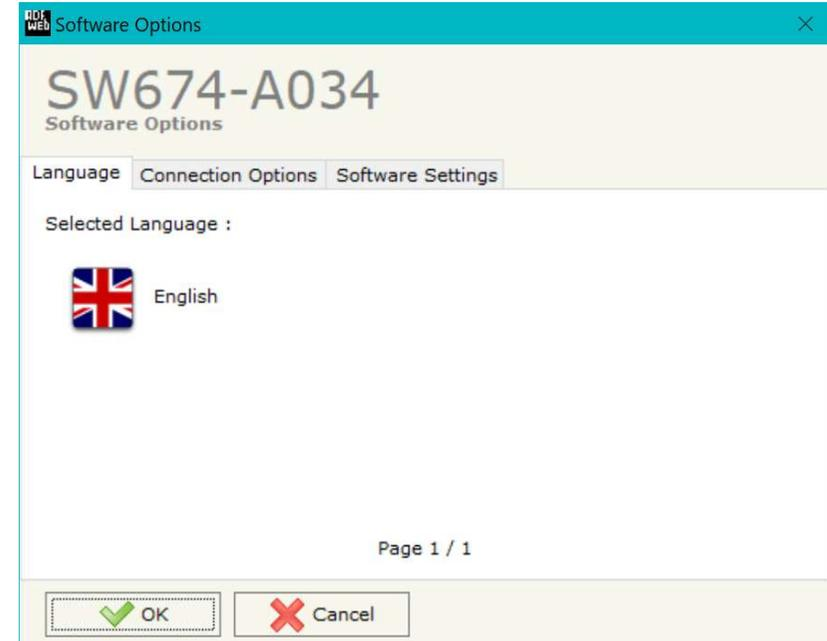
In the section “Connection Options”, it is possible to check if there are some updatings of the software compositor in ADFweb.com website. Checking the option “**Check Software Update at Start of Program**”, the SW674-A034 checks automatically if there are updatings when it is launched.
