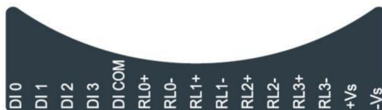
Figure 2.11 WISE-4060/LAN Pin Assignment
