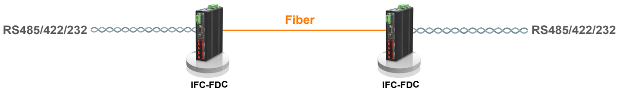
Figure 6 : Fiber Point to Point topology & application
