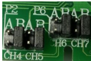
Thermistor: Pin B short
